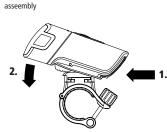
1. Put on the front headlight on rear edge of bracket 2. Press down until the front headlight engages in the clamp bracket 1. Press release button on underside and remove front headlamp (2.)
